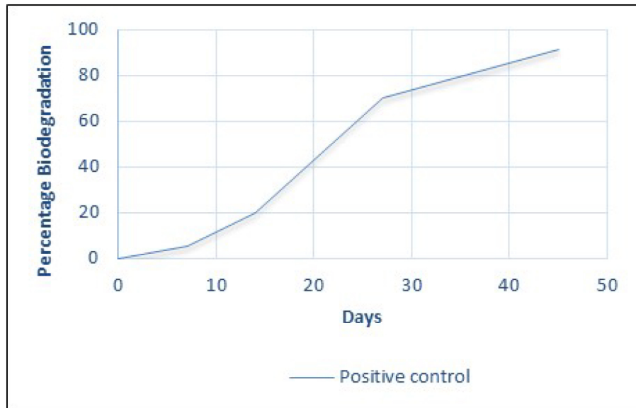
Graph 2a - The percent biodegradation of the positive control (reference material - cellulose) determined based on conversion of carbon from cellulose to carbon in the gaseous phase ( \text{CH}_4 and \text{CO}_2 )
